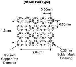
\* Dimensions are in millimeters.
