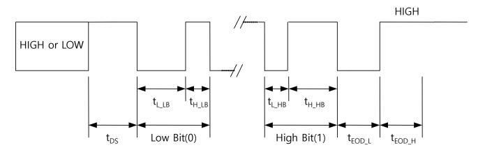
Figure 2. ExpressWire Interface - Bit Coding
