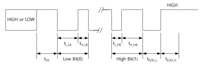
Figure 5. ExpressWire Interface - Bit Coding Time
