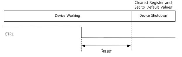
Figure 4. ExpressWire Interface – Set to Reset and Shutdown
