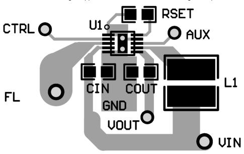
Figure 6. Recommended PCB Layout
