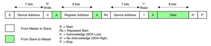
Figure 6. I<sup>2</sup>C Read Cycle
