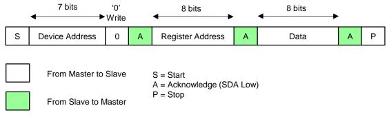
Figure 5. I<sup>2</sup>C Write Cycle
