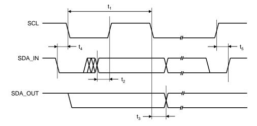
Figure 1. I<sup>2</sup>C Compatible Interface Timing
