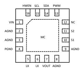
16-Lead 3mm x 3mm x 0.75mm TQFN Package
