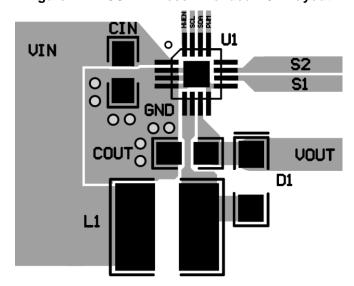
Figure 8. TQFN-16 Recommended PCB Layout
