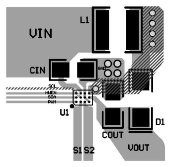
Figure 7. WLCSP-12 Recommended PCB Layout
