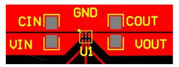
Figure 3. Recommended PCB Layout for WLCSP-9 Package
