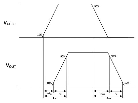
Figure 1. Timing Diagram
