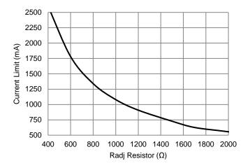
Figure 2. Current Limit Resistor Settings<sup>9</sup>
